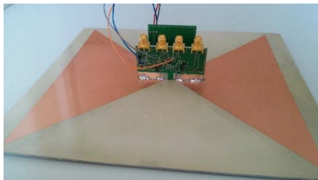
Fig. 7 Prototype of the short-dipole GPR front-end
