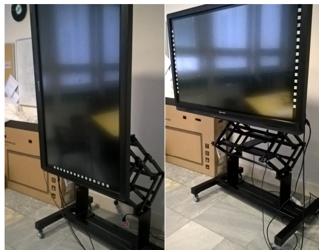
Fig. 3 Mount for a widescreen display with adjustable height and display rotation
