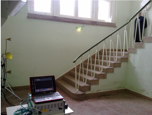
Fig. 4 Measurement location for line-of-sight measurement
