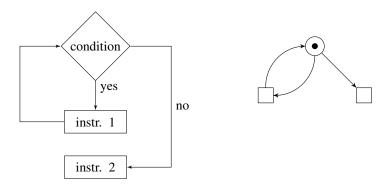
Fig. 3 Transcription of loop into ordinary Petri net
