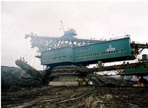
Fig. 3 RK 5000 Excavators at Mostecké uhelné Most equipped with the HFT system indicating ferromagnetic substances – result of the research team FA TUKE, SAS, developed and manufactured by EDIS Košice
