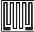
Fig. 5 The heater design based on conductive meander (line to gap thickness rate: 0,175/0,250 mm).
